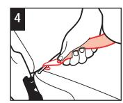
Fasten one LATCH belt hook to the anchor in the vehicle seat located in the vehicle seat bight. Repeat for other side of child restraint. See your vehicle owner's manual for locations and more information.
